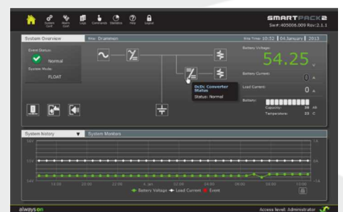
Status of DC/DC converters in Smartpack2 web
